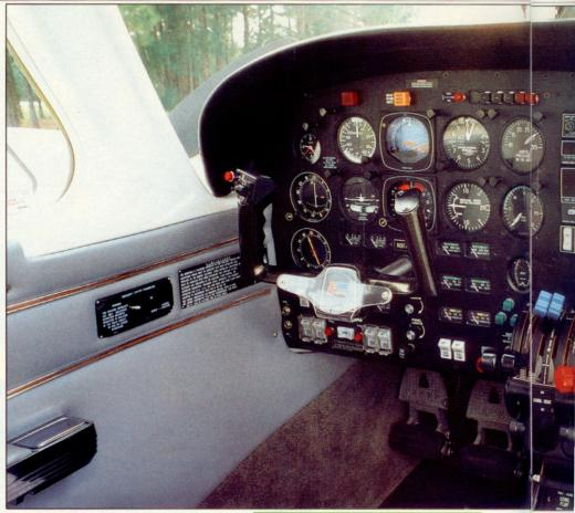
welcome change is the placement of the manifold pressure and propeller rpm gauges. They used to be on the pilot's subpanel, just above the right knee, where the pilot's view of them was obstructed by the control yoke. With the new Seminole, they are front and center, just to the right of the altimeter and vertical speed indicator.
