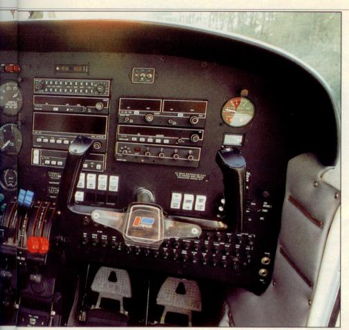
warning of low voltage in the electrical bus and another to signal overheating of the Janitrol heating unit. There is also a Hobbs meter for keeping track of the heater's time in service.
